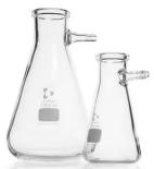
Separating chemicals (normally solid from liquid) by using a vacuum Dries solids after an experiment / lab
