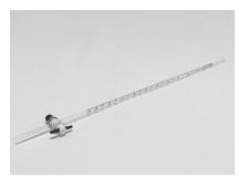
Distributing/Measuring a very precise amount of liquid, usually into a flask or beaker, during a chemical reaction
