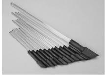
Stirring and mixing liquid mixtures Separating solids from liquids *rubber policeman*). Cleaning beakers/flasks
