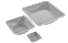
Container used to hold solids before adding them to liquids, or for weighing solids on a balance (mass)
